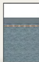
HALF WHITEBOARD PARTITION WITH TRUNKING
